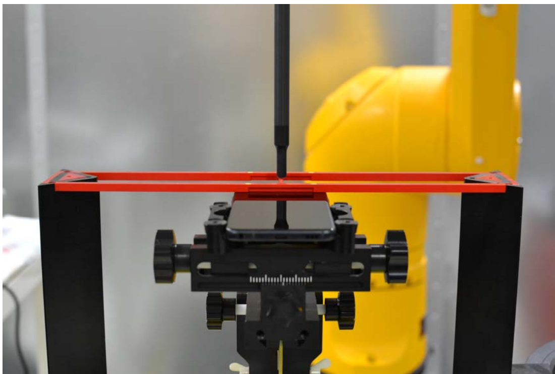
Figure 18-1 Ear Reference Point HAC Phantom Alignment
