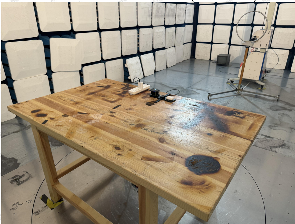
Photo of Radiation Emission Test (below 30MHz)
