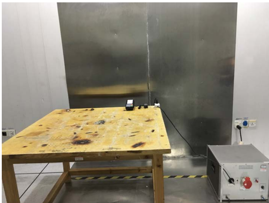
Photograph – Conducted Emission Test Setup
