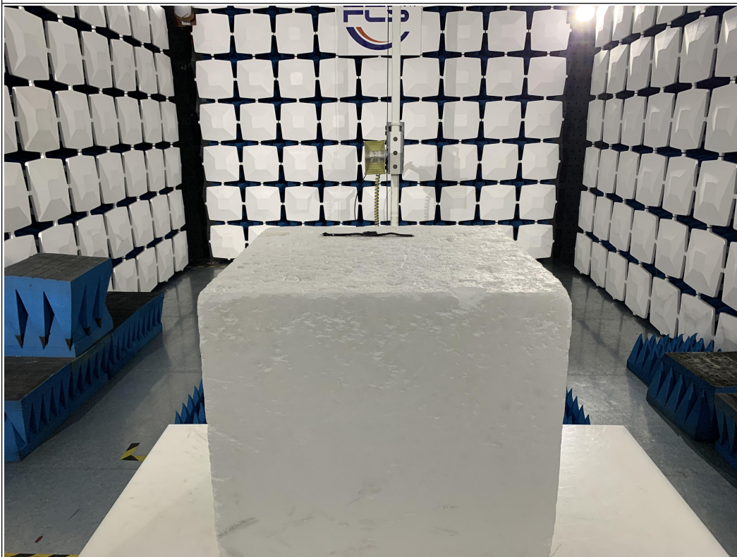
Above 1GHz for radiated emission test setup
