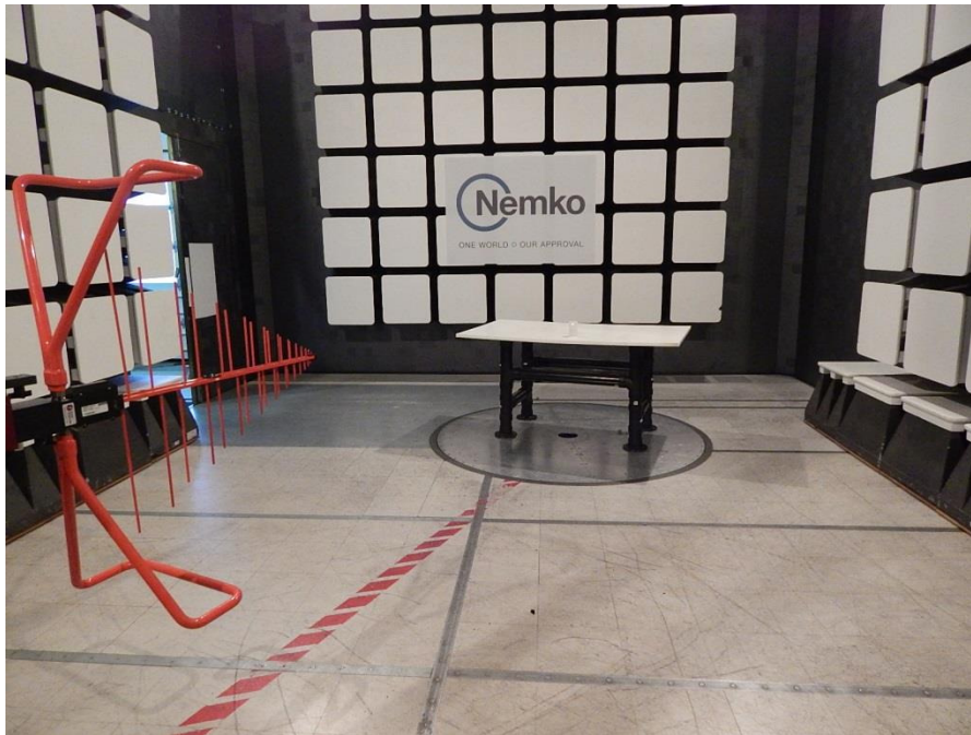
Figure 8.2-1: Radiated emissions setup photo – 30 to 1000 MHz
