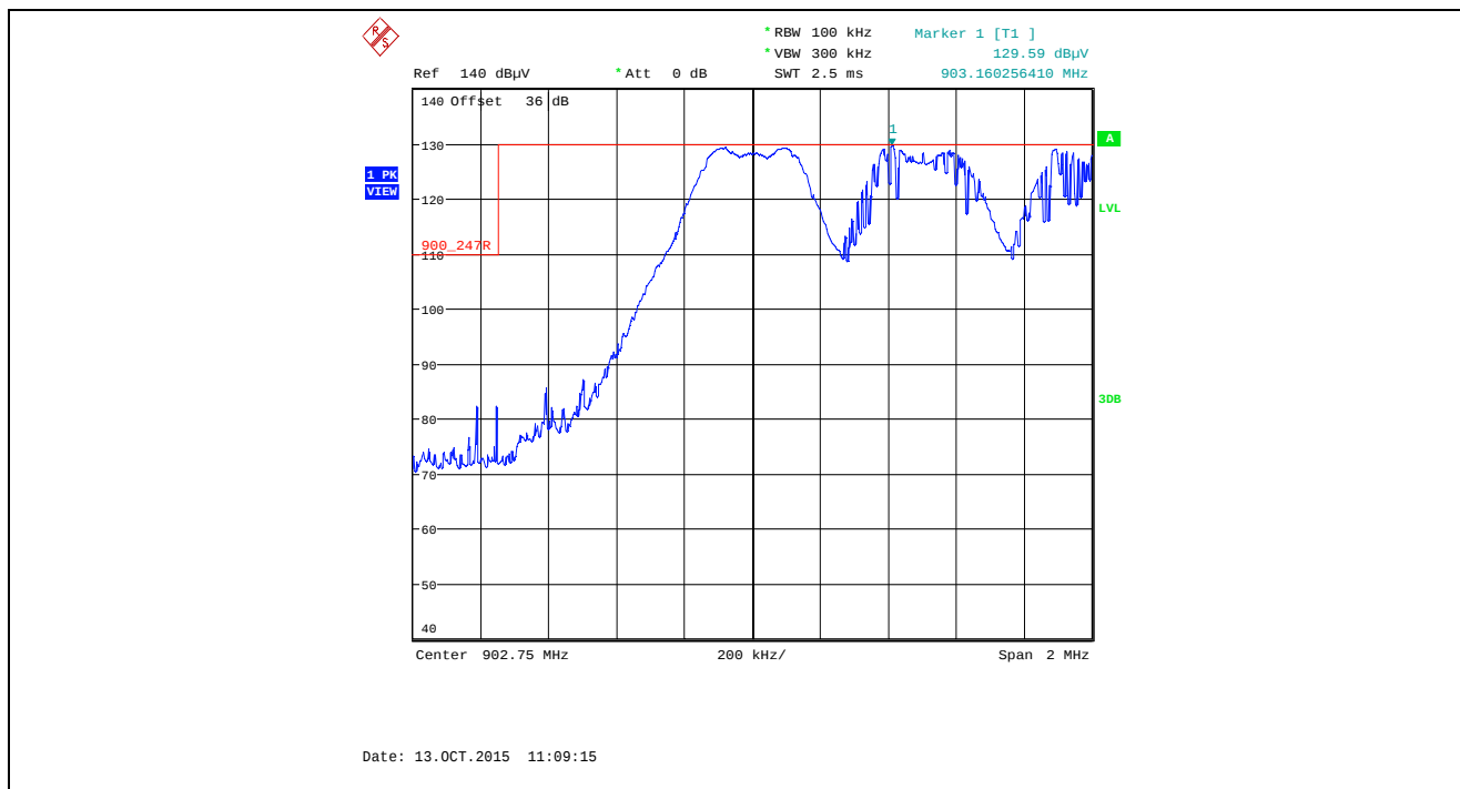
Plot 5.5.4.1.2.20. Band-Edge RF Radiated Emissions at 3 m, Vertical Polarization Pseudorandom Hopping Mode, Low End of Frequency Band, 902.75 MHz, XB2, Data Rate at 250 kbps
