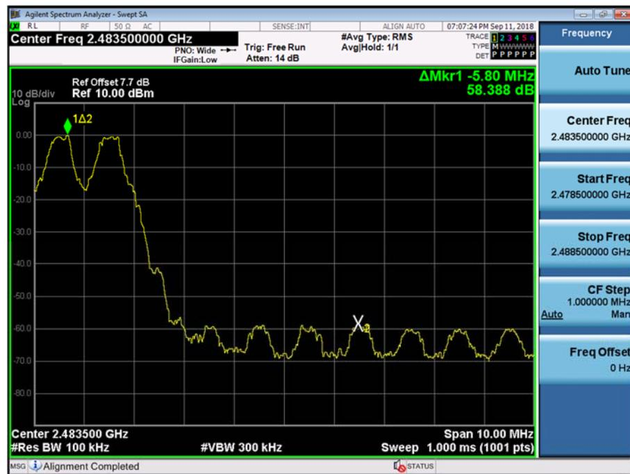
Test Plots with hopping (8DPSK)
