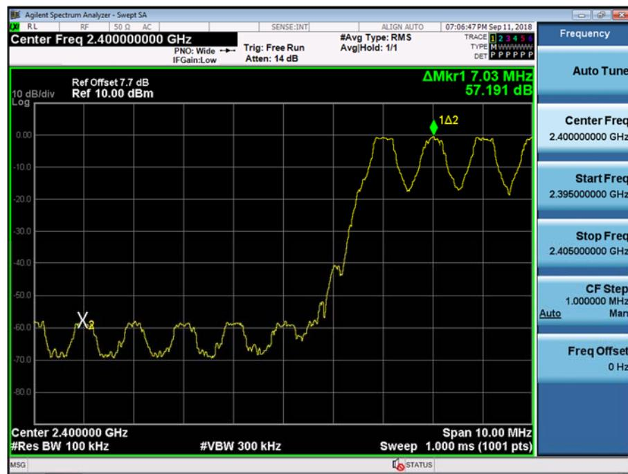
Test Plots with hopping (GFSK)
