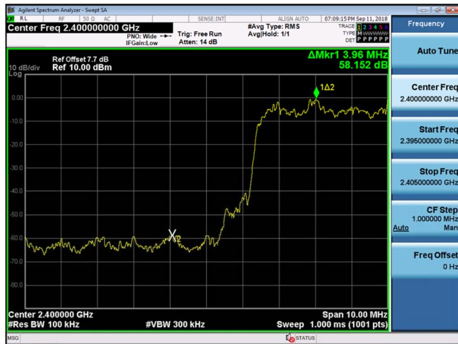
Test Plots with hopping (8DPSK)
