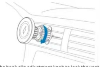
Turn the hook clip adjustment knob to lock the vent blade tightly.
