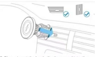
Please insert the hook clip downward into the vent blade. This product is suitable for all horizontal and vertical vents.
