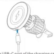
Insert the USB-C port of the charging cable into the bottom of the product. Plug the USB-A port into the car charger (QC 3.0 / 9V-2A minimum required).
