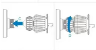
Carefully follow the steps to assemble the product. Note: the direction of the nut can not be wrong. To insert with force, make sure the ball joint inserted into the bolt.
