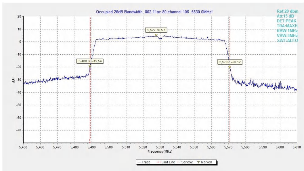
Fig.31 Occupied 26dB Bandwidth (802. 11ac-HT80, 5530MHz)
