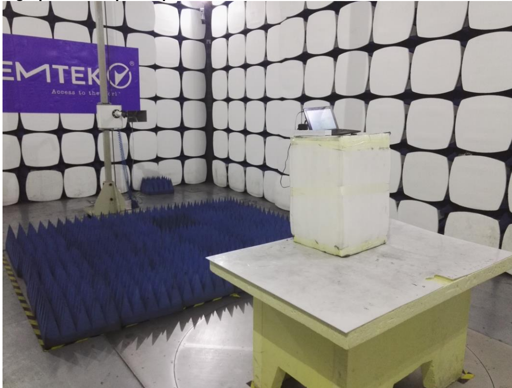
Photograph 4: Set-up for Spurious Emissions for 18 - 26.5GHz
