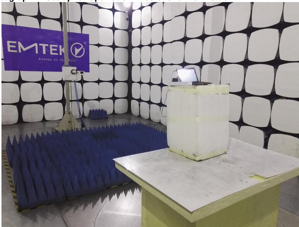
Photograph 4: Set-up for Spurious Emissions for 18 - 26.5GHz
