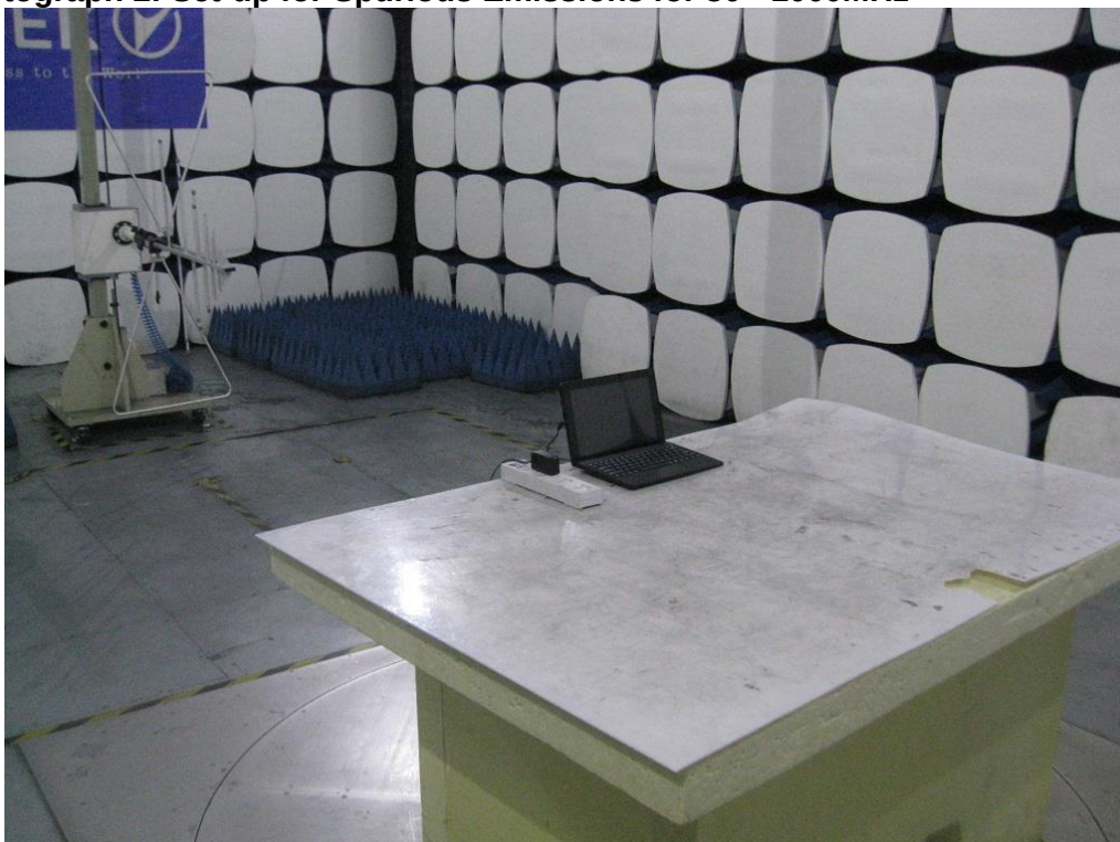
Photograph 2: Set-up for Spurious Emissions for 30 - 1000MHz
