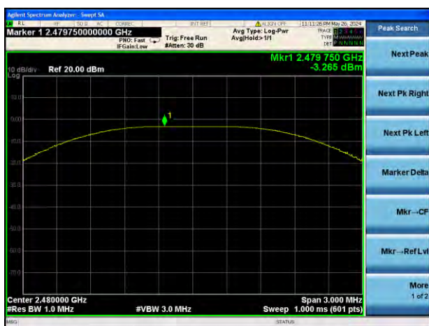
GFSK (BLE 1Mbps) HIGH CHANNEL
