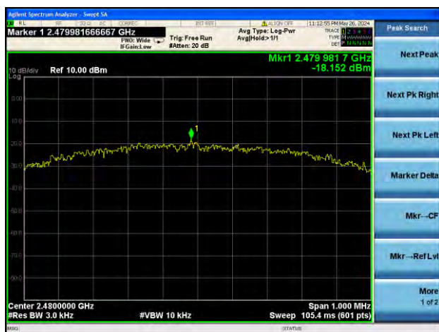
GFSK (BLE 1Mbps) HIGH CHANNEL
