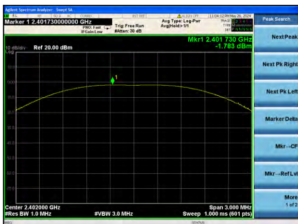
GFSK (BLE 1Mbps) LOW CHANNEL
