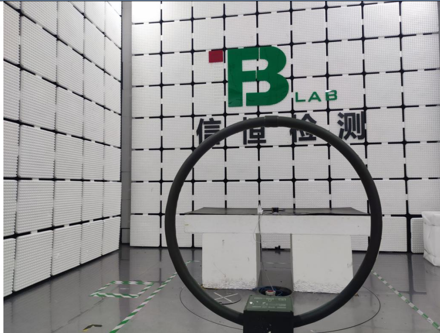
Radiated Emission (9 kHz -30MHz)
