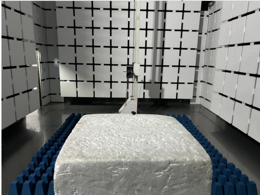
Radiated Emissions (above 1GHz) R-ear
