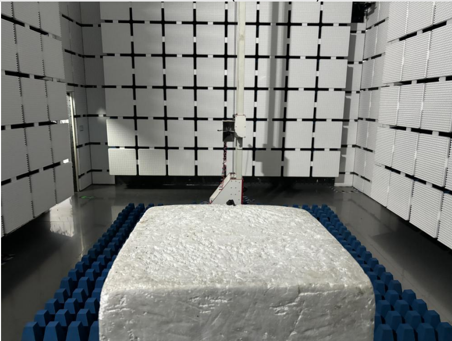
Radiated Emissions (above 1GHz) L-ear
