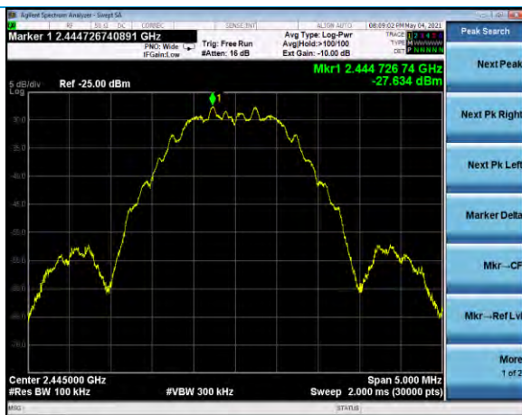
Neg40dBm, channel 19, reference plot -27.6 dBm
