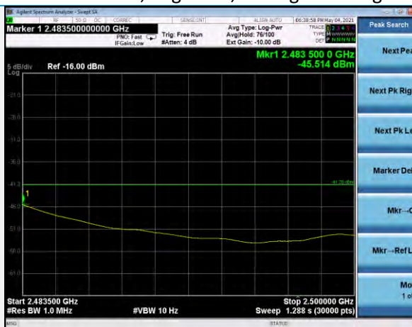
2.4835-2.5 GHz, Terminated Method, 10 Hz RBW Channel 25, neg4dBm, Average Reading
