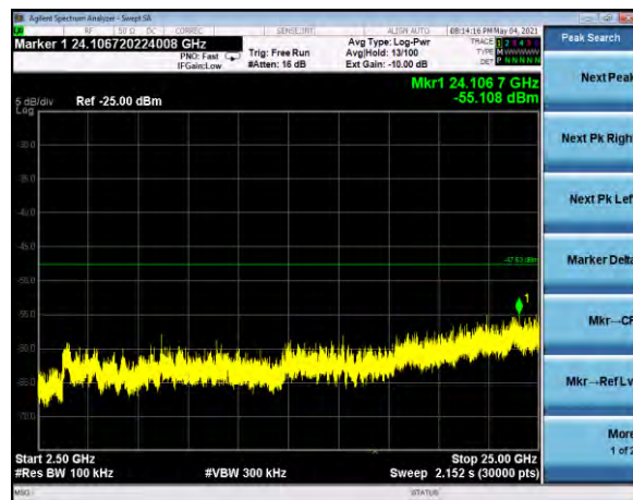
Conducted TX Spurious 2.5-25 GHz Channel 19, neg40dBm
