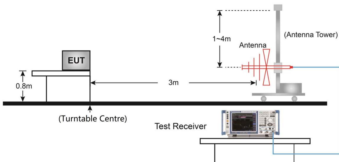
Above 1GHz Test Setup:
