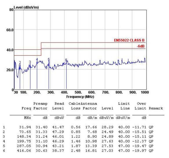
Test mode: TX Mode Polarization: HORIZONTAL
