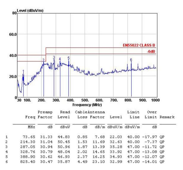
Test mode: 2402MHz Polarization: VERTICAL
