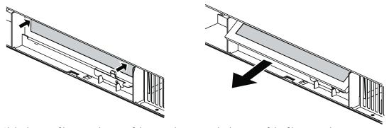
5 Slide the new filter into the top of the unit, then press the bottom of the filter into place.
