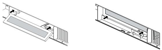
**6** Carefully push the vent grille back into place and replace the vent grille mounting screws.
