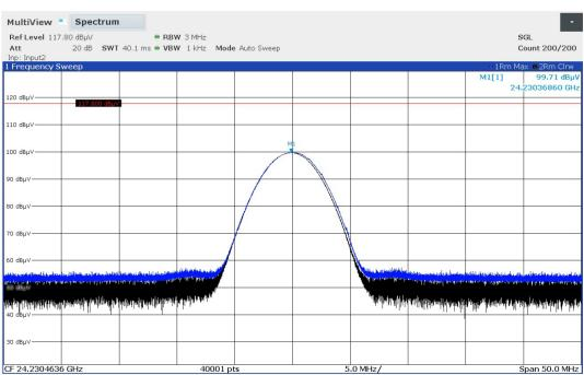
Note: The resolution bandwidth was set greater than occupied bandwidth of fundamental.
