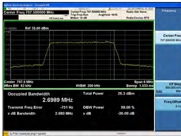
Band12 / 3MHz / High CH / QPSK
