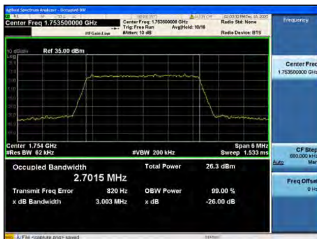
Band4 / 3MHz / High CH / QPSK
