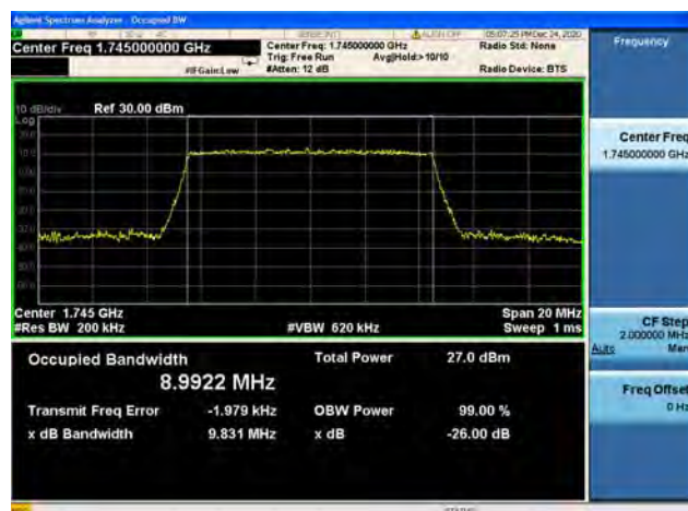
Band66 / 10MHz / High CH / QPSK
