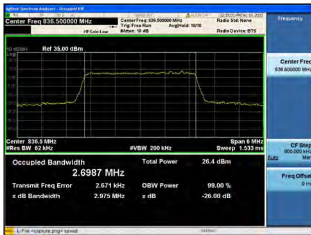
Band5 / 3MHz / High CH / QPSK
