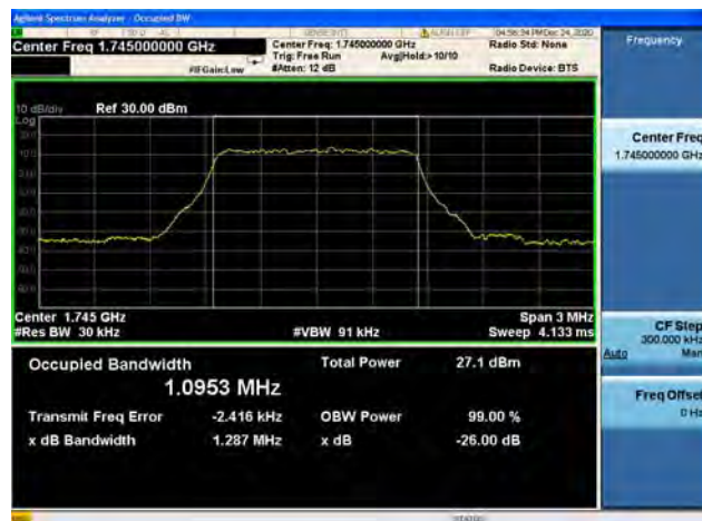
Band66 / 1.4MHz / High CH / QPSK
