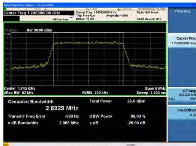
Band66 / 3MHz / High CH / QPSK
