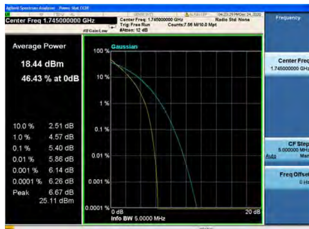
Band66 / 5MHz / High CH / QPSK
