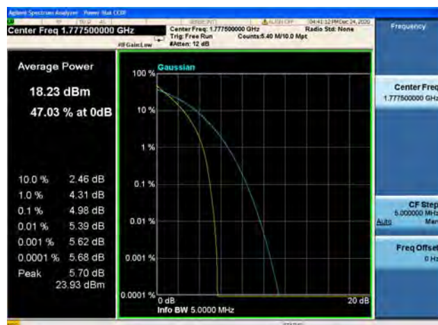
Band66 / 5MHz / High CH / QPSK
