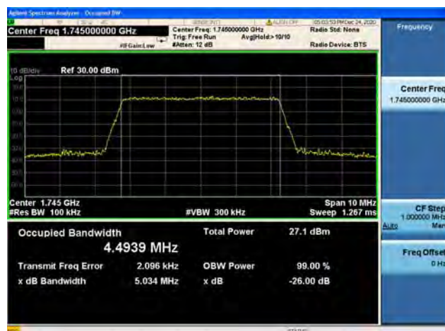
Band66 / 5MHz / High CH / QPSK
