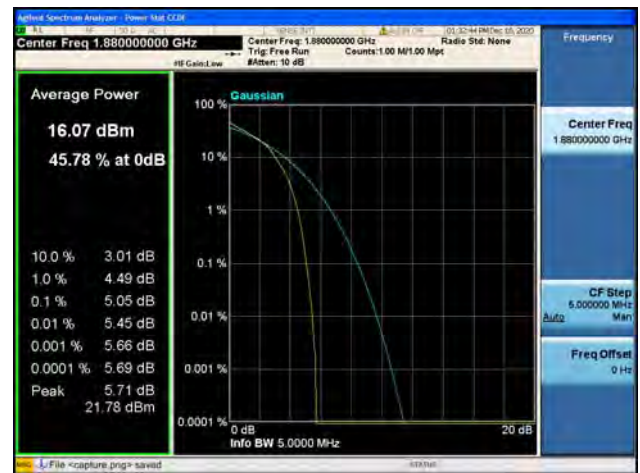
Band2 / 3MHz / High CH / 16QAM
