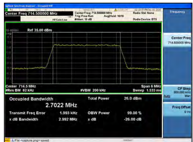
Band12 / 3MHz / High CH / 16QAM
