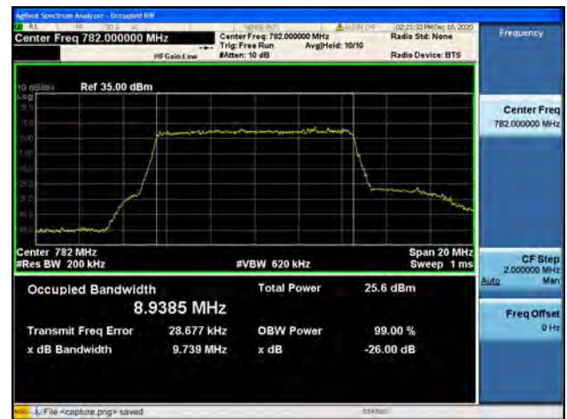
Band13 / 10MHz / High CH / 16QAM
