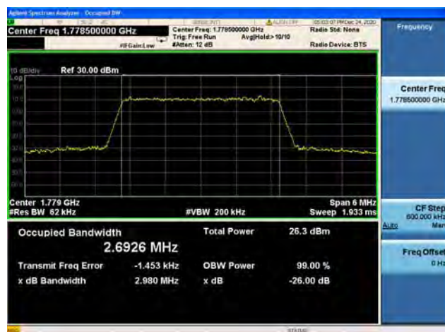
Band66 / 3MHz / High CH / QPSK
