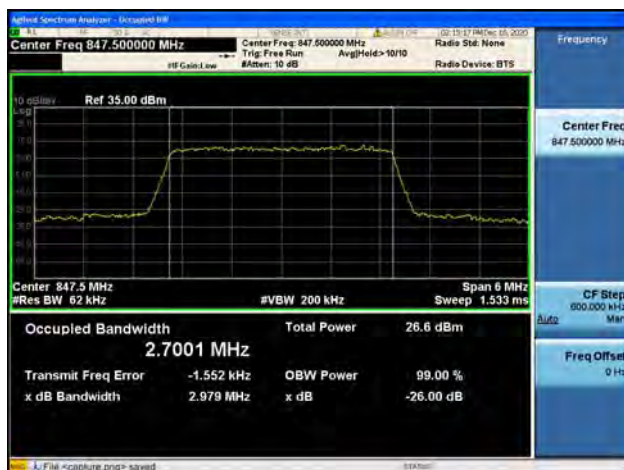
Band5 / 3MHz / High CH / QPSK
