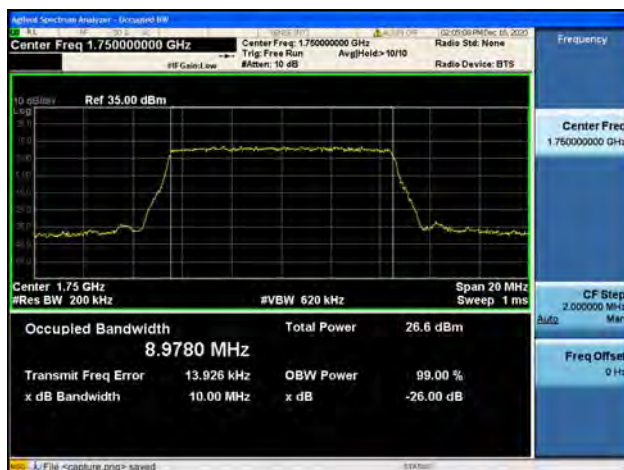
Band4 / 10MHz / High CH / QPSK
