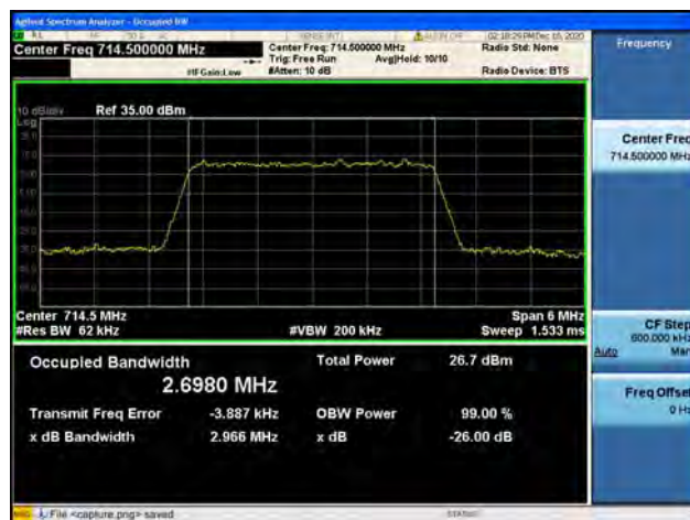
Band12 / 3MHz / High CH / QPSK
