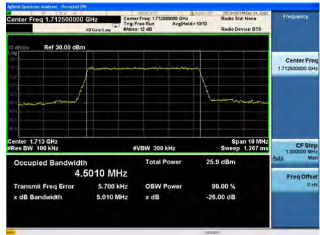
Band66 / 5MHz / Mid CH / 16QAM
