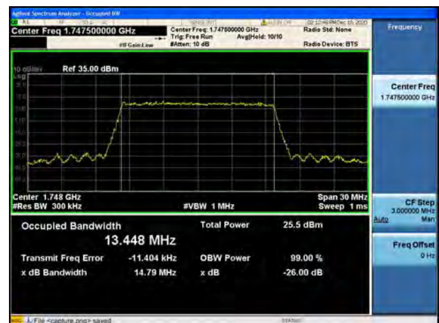
Band4 / 15MHz / High CH / 16QAM
