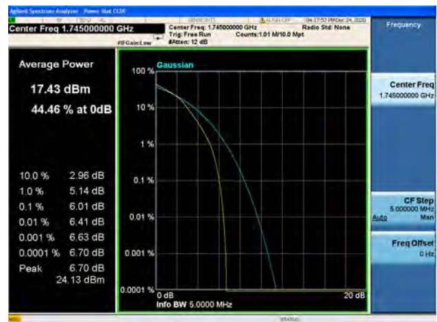
Band66 / 3MHz / High CH / 16QAM
