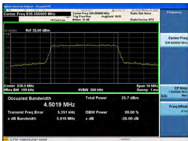
Band5 / 5MHz / High CH / 16QAM
