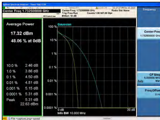
Band4 / 10MHz / High CH / QPSK
