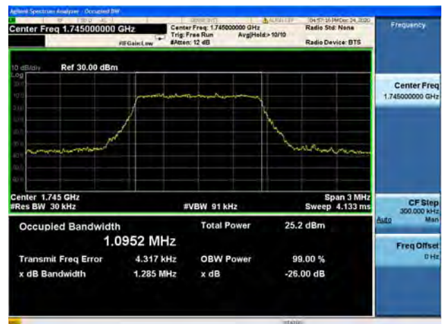
Band66 / 1.4MHz / High CH / 16QAM
