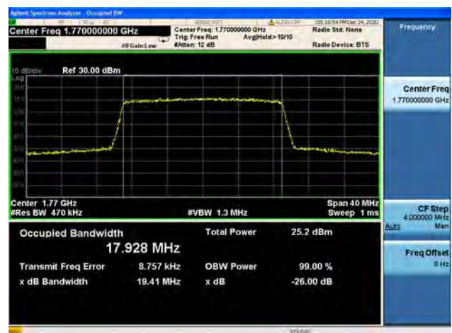
Band66 / 20MHz / High CH / 16QAM
