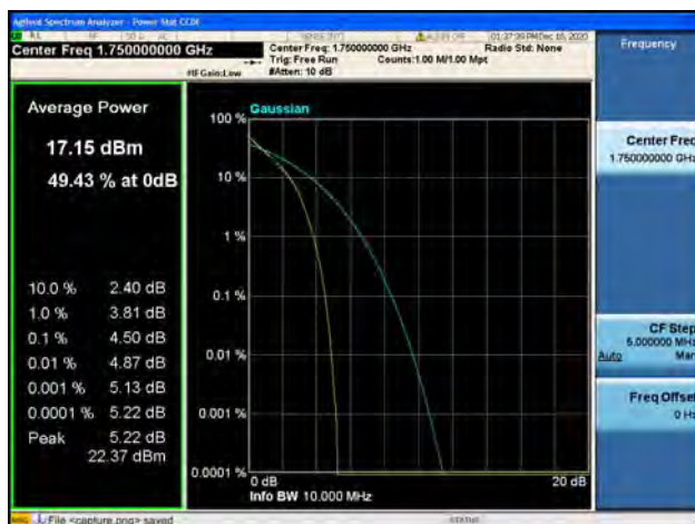
Band4 / 10MHz / High CH / QPSK
