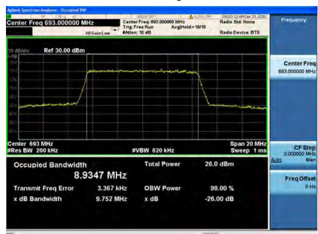
Band71 / 10MHz / High CH / 16QAM
