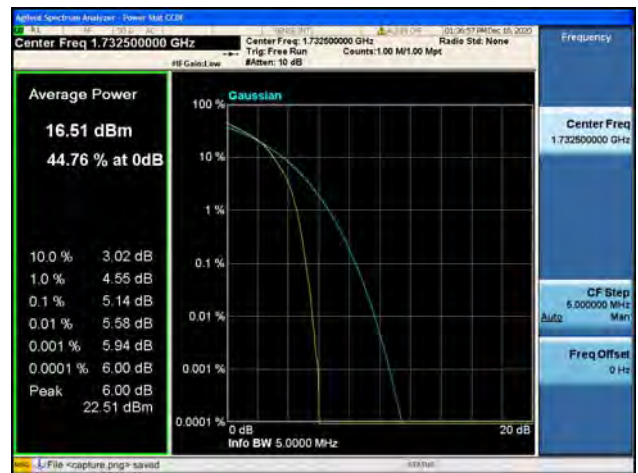
Band4 / 5MHz / High CH / 16QAM
