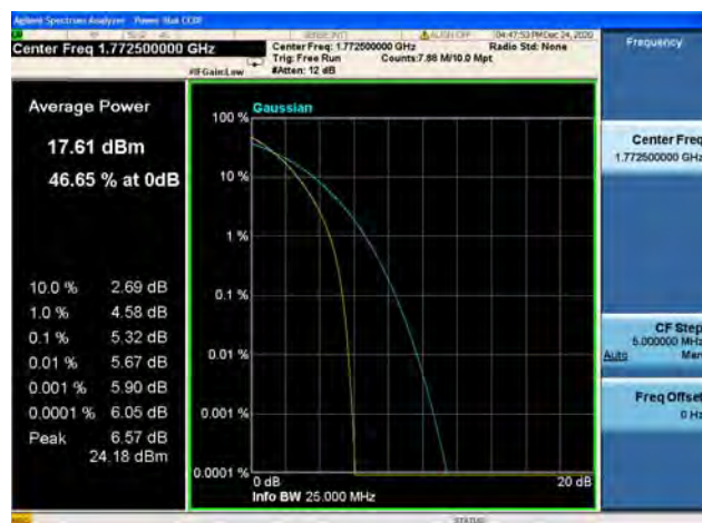
Band66 / 15MHz / High CH / QPSK
