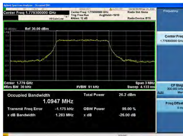
Band66 / 1.4MHz / High CH / QPSK
