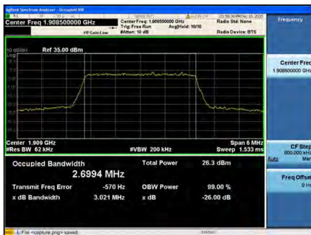
Band2 / 3MHz / High CH / QPSK
