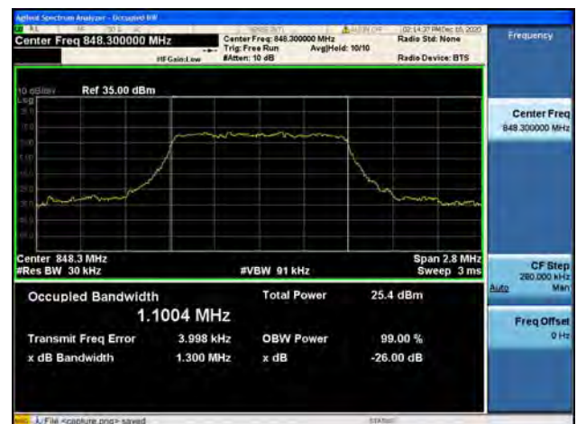
Band5 / 1.4MHz / High CH / 16QAM
