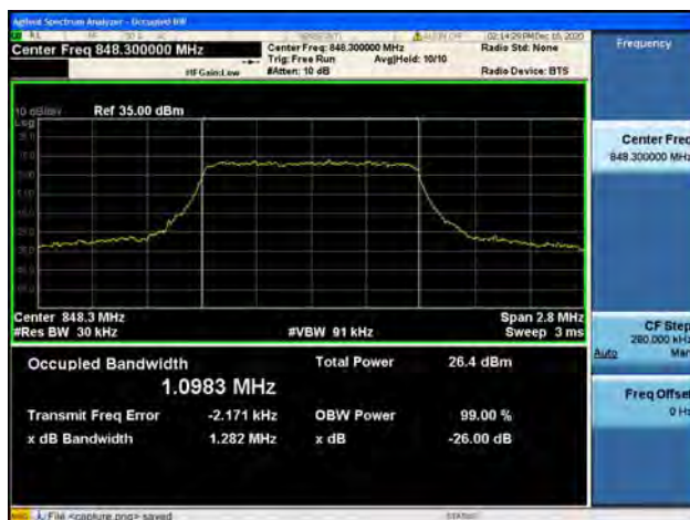
Band5 / 1.4MHz / High CH / QPSK
