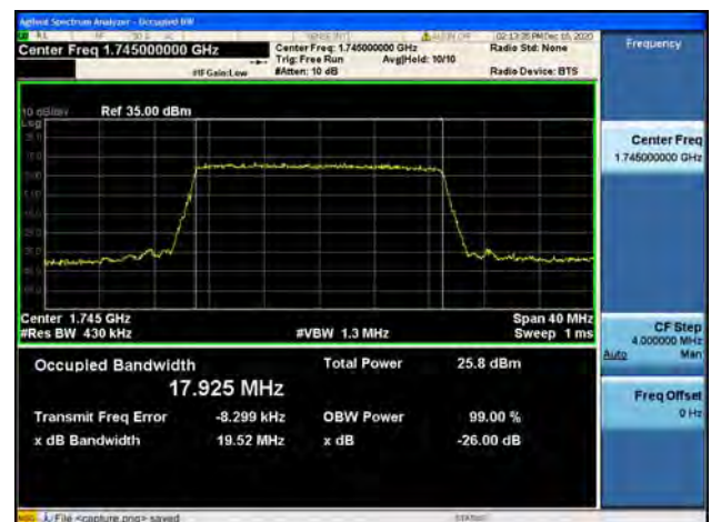
Band4 / 20MHz / High CH / 16QAM
