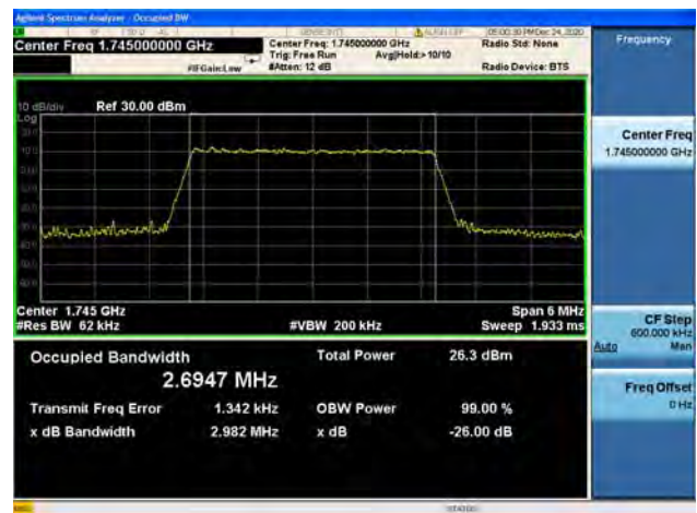
Band66 / 3MHz / High CH / 16QAM
