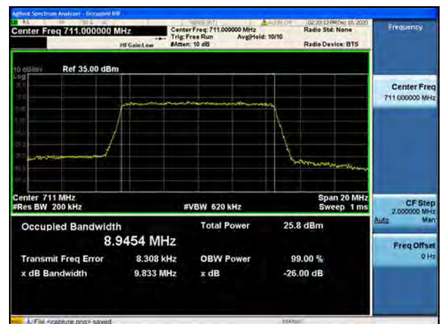
Band12 / 10MHz / High CH / 16QAM
