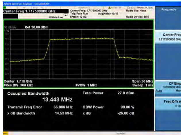
Band66 / 15MHz / Mid CH / QPSK
