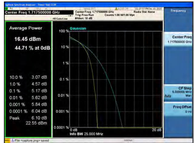
Band4 / 15MHz / Mid CH / 16QAM
