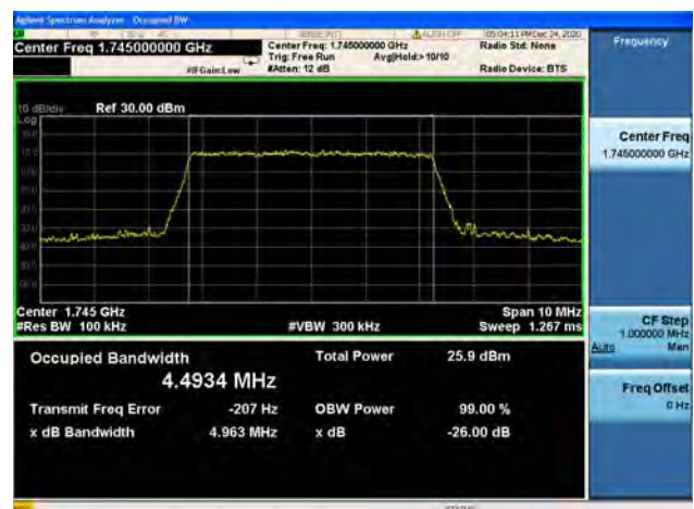
Band66 / 5MHz / High CH / 16QAM
