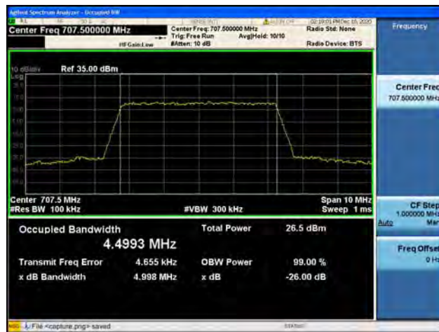
Band12 / 5MHz / High CH / QPSK
