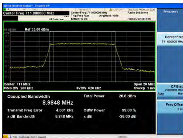
Band12 / 10MHz / High CH / QPSK
