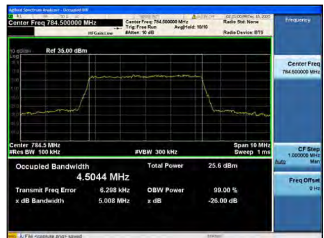
Band13 / 5MHz / High CH / 16QAM
