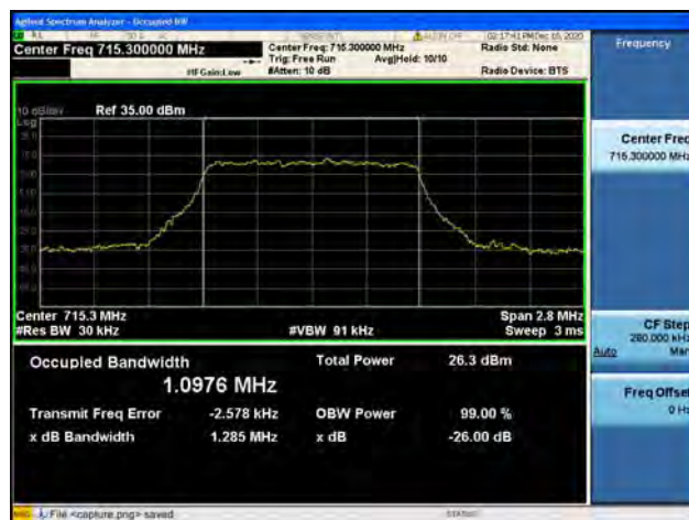
Band12 / 1.4MHz / High CH / QPSK
