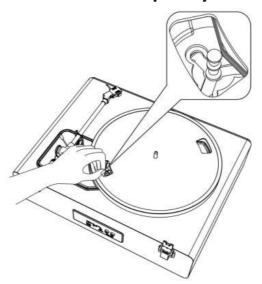
3. Remove the main platter and then remove the old belt.
