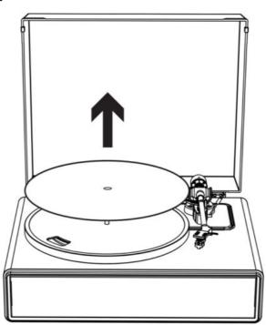
2. Remove the belt from the motor pulley.
