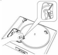
7. Using your hands, slowly rotate the platter ten times in a clockwise direction as shown by the arrow below.
