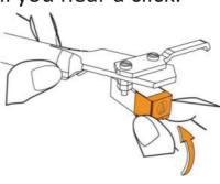
3. Make sure there is no gap between the headshell and the cartridge.
