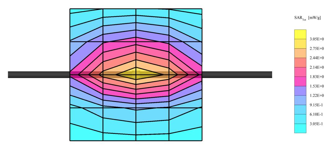
SAM 1 (Cellular - Brain Tissue) Frequency: 835 MHz; Crest factor: 1.0 Validation 835MHz - Brain Tissue:  $\sigma = 0.92$  mho/m  $\epsilon_r = 41.5 \rho = 1.00$  g/cm<sup>3</sup> Probe: ET3DV6 - SN1505; ConvF(7.00,7.00,7.00) Cubes (2): Peak: 3.66 mW/g  $\pm$  0.06 dB, SAR (1g): 2.44 mW/g  $\pm$  0.06 dB, SAR (10g): 1.59 mW/g  $\pm$  0.06 dB, (Advanced extrapolation) Penetration depth: 12.9 (12.3, 13.7) [mm] Powerdrift: 0.00 dB Liquid Temperature (°C): 21.4
