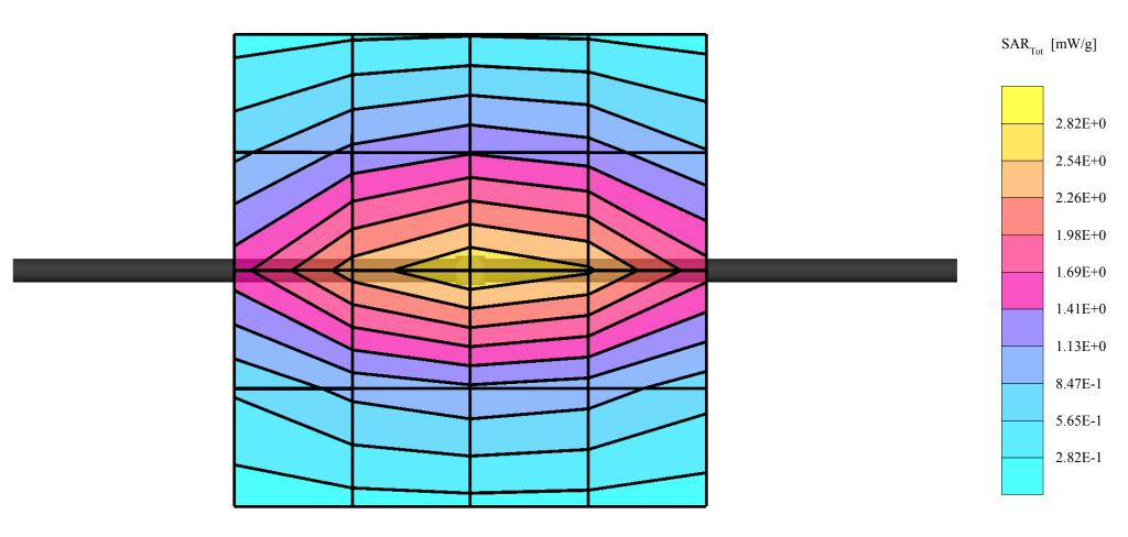
SAM 1 (Cellular - Brain Tissue) Frequency: 835 MHz; Crest factor: 1.0 Validation 835MHz - Brain Tissue:  $\sigma = 0.92$  mho/m  $\varepsilon_r = 40.9 \ \rho = 1.00 \ g/cm^3$ Probe: ET3DV6 - SN1505; ConvF(7.00,7.00,7.00) Cubes (2): Peak: 3.69 mW/g  $\pm$  0.03 dB, SAR (1g): 2.47 mW/g  $\pm$  0.04 dB, SAR (10g): 1.62 mW/g  $\pm$  0.04 dB, (Advanced extrapolation) Penetration depth: 13.0 (12.5, 13.7) [mm] Powerdrift: -0.01 dB Liquid Temperature (°C): 21.5
