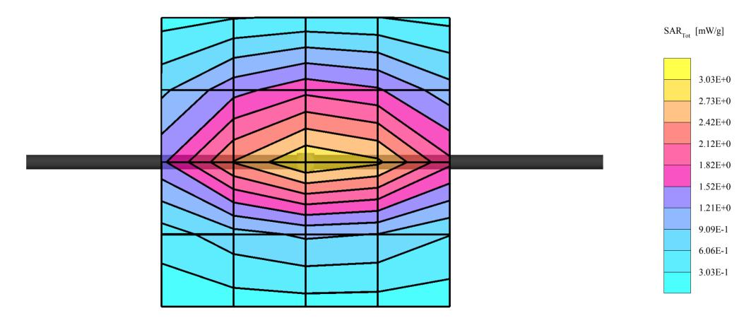
SAM 1 (Cellular - Brain Tissue) Phantom Frequency: 900 MHz; Crest factor: 1.0 Validation 900MHz - Brain Tissue:  $\sigma = 1.00$  mho/m  $\varepsilon_r = 39.5 \ \rho = 1.00$  g/cm<sup>3</sup> Probe: ET3DV6 - SN1504; ConvF(6.50,6.50,6.50) Cubes (2): SAR (1g): 3.03 mW/g  $\pm$  0.06 dB, SAR (10g): 1.88 mW/g  $\pm$  0.06 dB, (Worst-case extrapolation) Coarse: Dx = 20.0, Dy = 20.0, Dz = 10.0 Powerdrift: -0.18 dB Liquid Temperature (°C): 20.6
