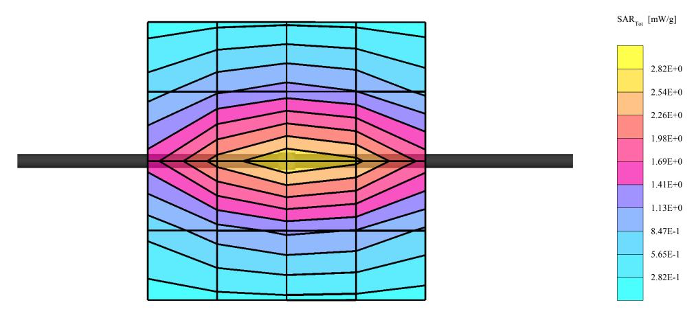
SAM 2 (Cellular - Muscle Tissue) Phantom Frequency: 835 MHz; Crest factor: 1.0 Validation 835MHz - Muscle Tissue:  $\sigma = 0.95$  mho/m  $\varepsilon_r = 54.9 \ \rho = 1.00 \ g/cm^3$ Probe: ET3DV6 - SN1504; ConvF(6.50,6.50,6.50) Cubes (2): SAR (1g): 2.70 mW/g  $\pm$  0.06 dB, SAR (10g): 1.75 mW/g  $\pm$  0.06 dB, (Worst-case extrapolation) Coarse: Dx = 20.0, Dy = 20.0, Dz = 10.0 Powerdrift: -0.17 dB Liquid Temperature (°C): 20.5
