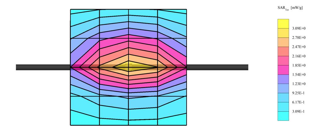
SAM 1 (Cellular - Brain Tissue) Frequency: 900 MHz; Crest factor: 1.0 Validation 900MHz - Brain Tissue:  $\sigma = 1.00$  mho/m  $\varepsilon_r = 39.8 \ \rho = 1.00$  g/cm<sup>3</sup> Probe: ET3DV6 - SN1504; ConvF(6.50,6.50,6.50) Cubes (2): Peak: 4.87 mW/g ± 0.08 dB, SAR (1g): 2.98 mW/g ± 0.08 dB, SAR (10g): 1.85 mW/g ± 0.07 dB, (Worst-case extrapolation) Penetration depth: 11.0 (9.9, 12.5) [mm] Powerdrift: -0.20 dB Liquid Temperature (°C): 20.5
