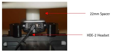
Note: the 22mm spacer was removed before the SAR measurement.
