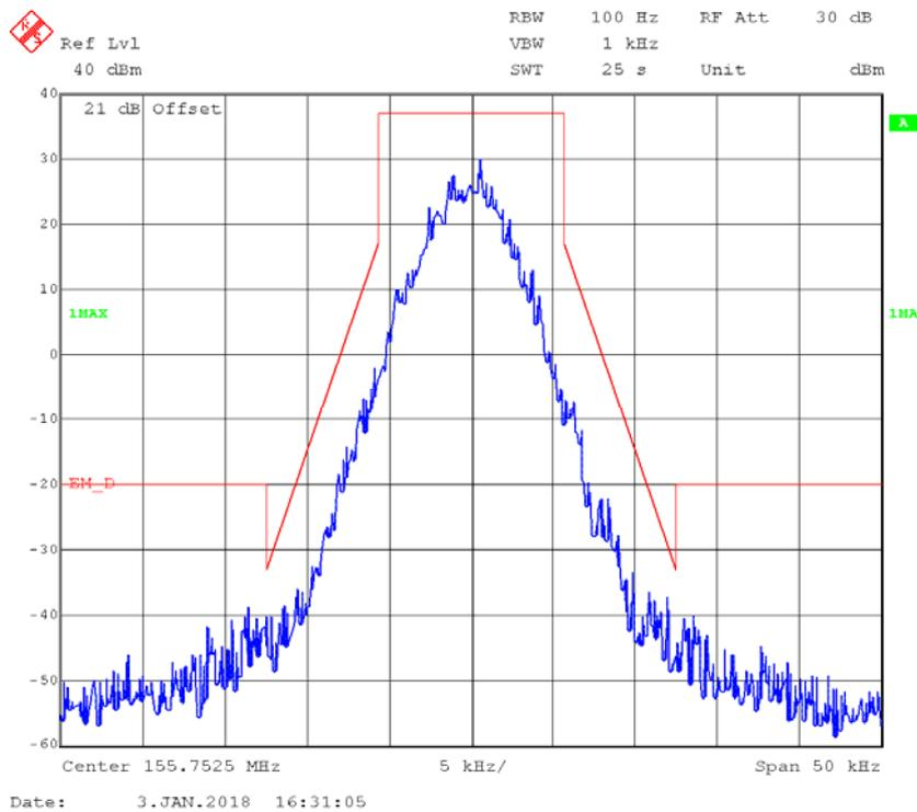
**4FSK,12.5kHz,Low Power - Frequency 155.7525 MHz: 99% Occupied & 26 dB Bandwidth**
