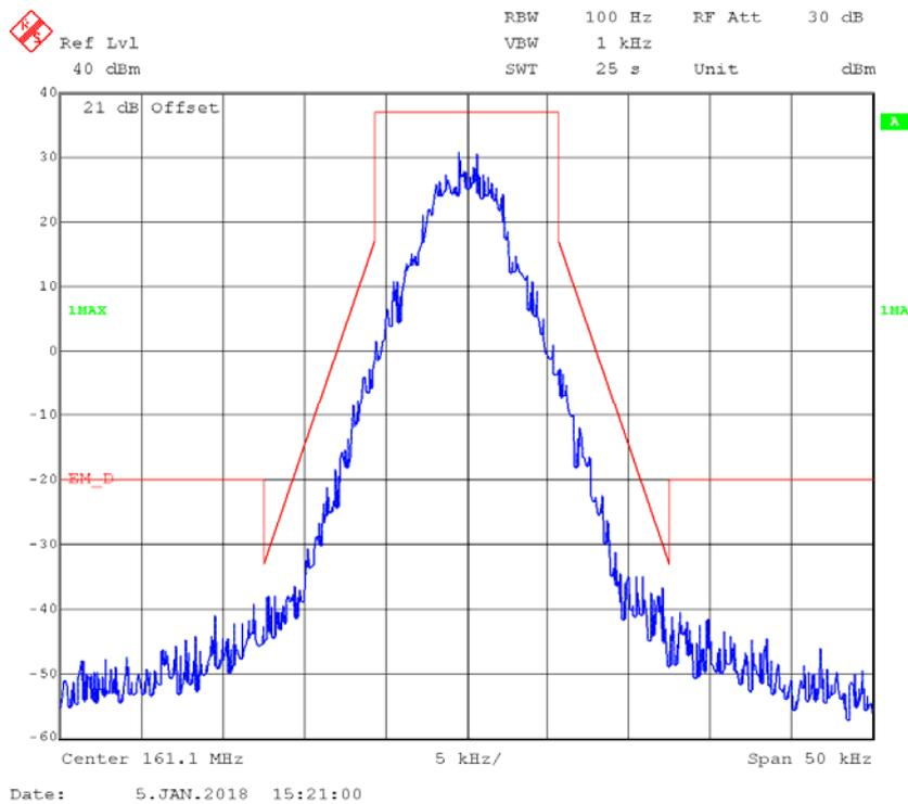
**4FSK,12.5kHz,Low Power - Frequency 161.1 MHz: 99% Occupied & 26 dB Bandwidth**
