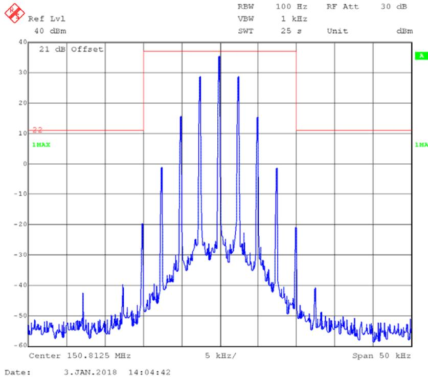
**FM,12.5kHz,Low Power - Frequency 150.8125 MHz: 99% Occupied & 26 dB Bandwidth**
