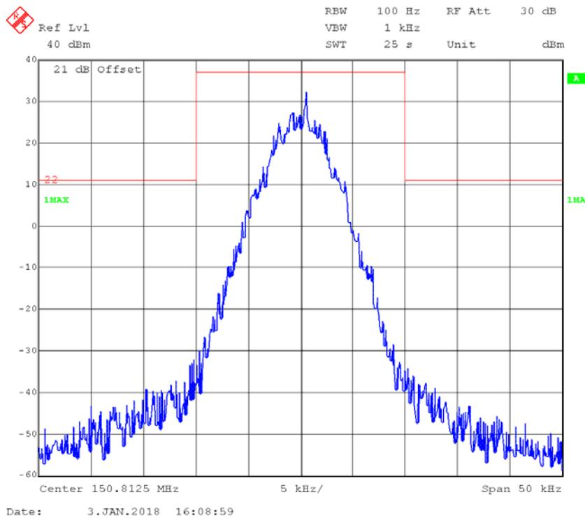
**4FSK,12.5kHz,Low Power - Frequency 150.8125 MHz: 99% Occupied & 26 dB Bandwidth**
