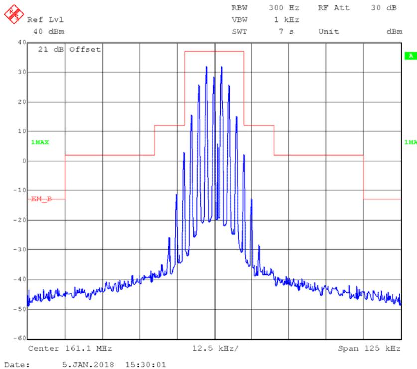
**4FSK,12.5kHz,High Power - Frequency 161.1 MHz: 99% Occupied & 26 dB Bandwidth**
