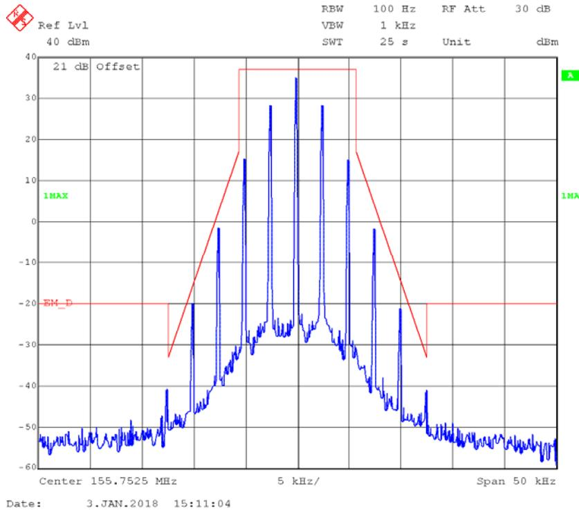
**FM,12.5kHz,Low Power - Frequency 155.7525 MHz: 99% Occupied & 26 dB Bandwidth**
