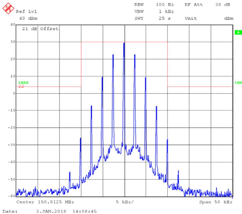
**FM,25kHz,High Power - Frequency 150.8125 MHz: 99% Occupied & 26 dB Bandwidth**
