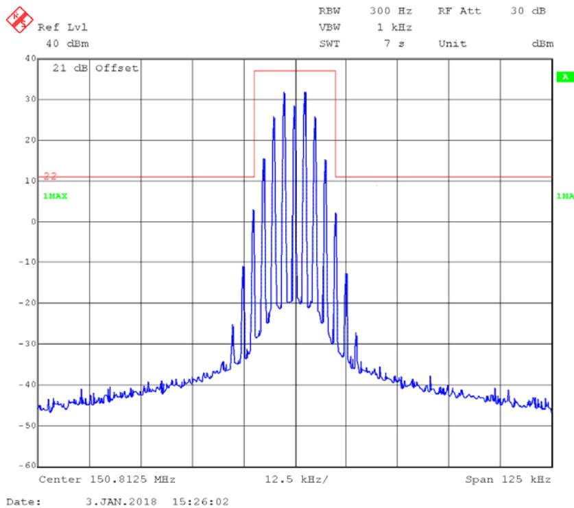
**FM,25kHz,Low Power - Frequency 150.8125 MHz: 99% Occupied & 26 dB Bandwidth**
