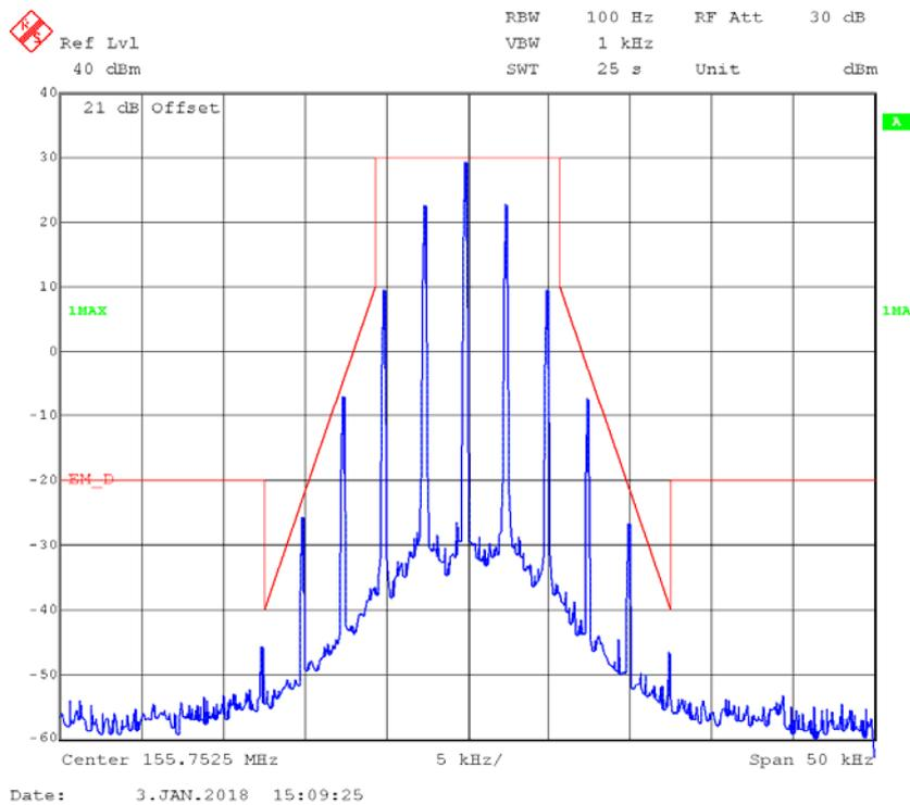
**4FSK,12.5kHz,High Power - Frequency 155.7525 MHz: 99% Occupied & 26 dB Bandwidth**
