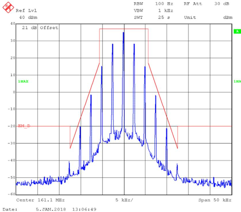
**FM,12.5kHz,Low Power - Frequency 161.1 MHz: 99% Occupied & 26 dB Bandwidth**
