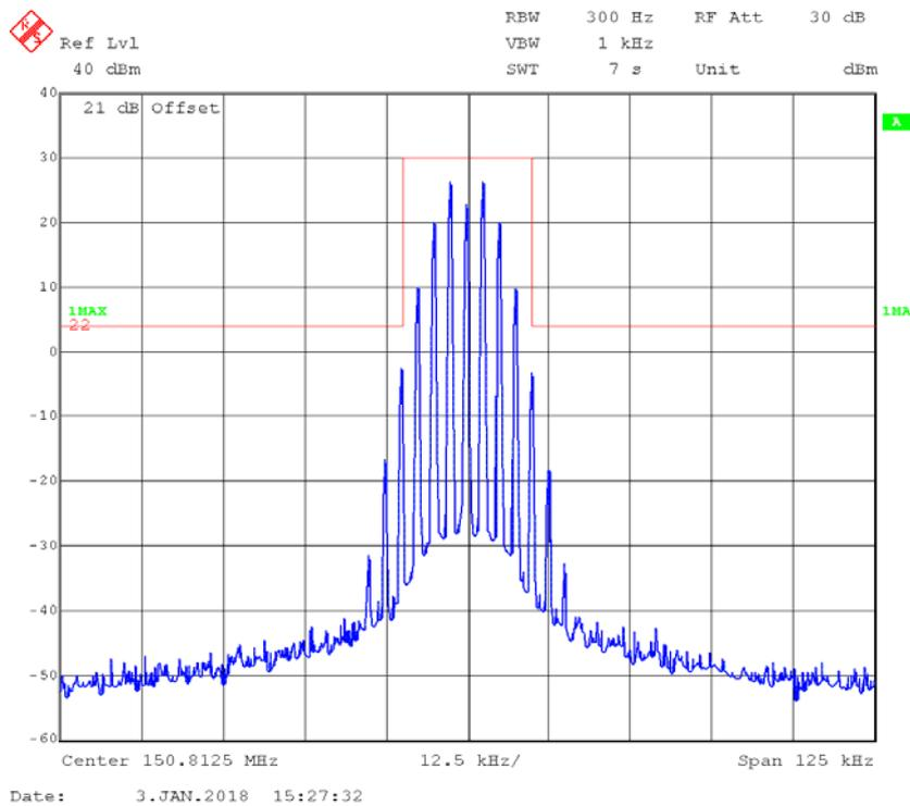
**4FSK,12.5kHz,High Power - Frequency 150.8125 MHz: 99% Occupied & 26 dB Bandwidth**
