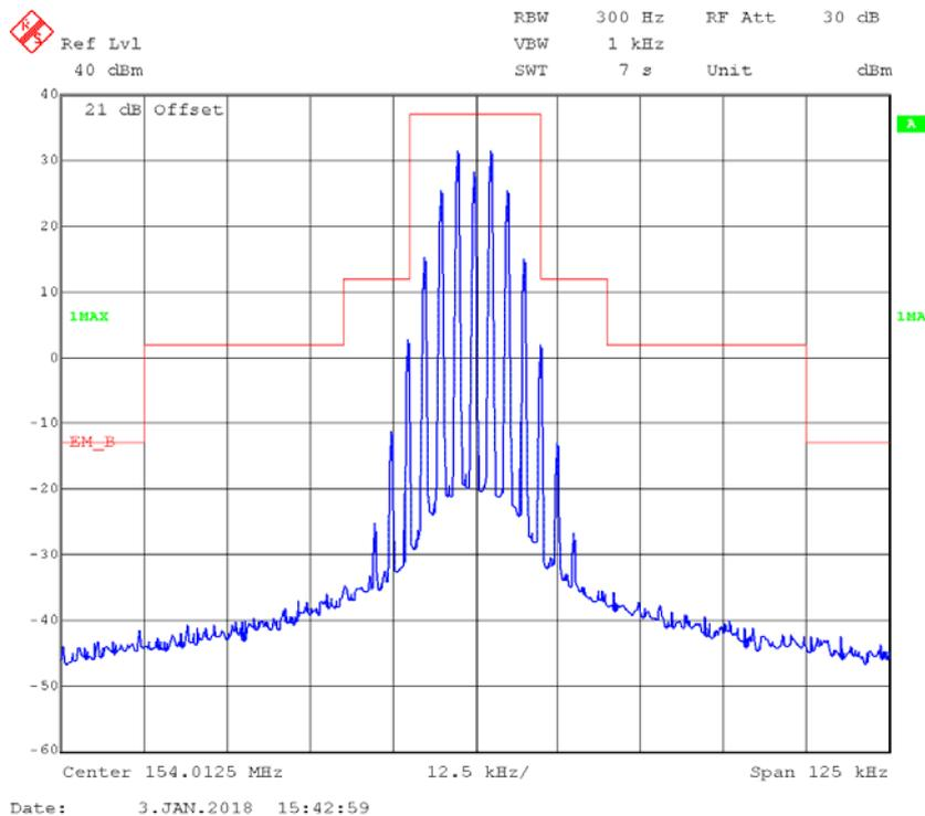
**FM,25kHz,Low Power - Frequency 154.0125 MHz MHz: 99% Occupied & 26 dB Bandwidth**
