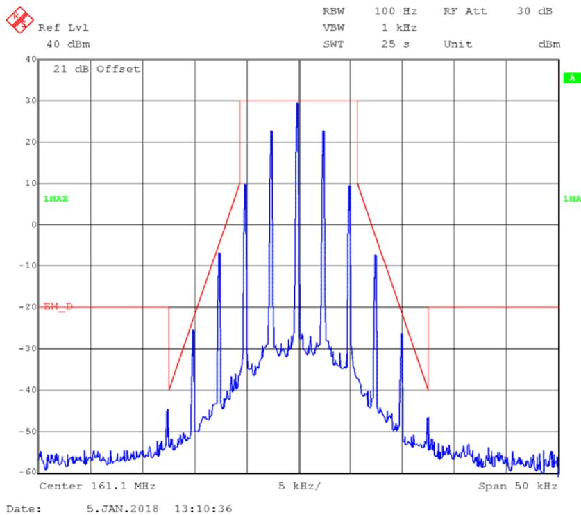
**FM,25kHz,High Power - Frequency 161.1 MHz: 99% Occupied & 26 dB Bandwidth**
