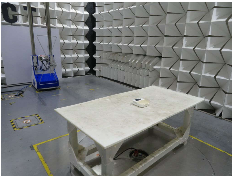
Radiated spurious emission Test Setup-2(Below 1GHz)
