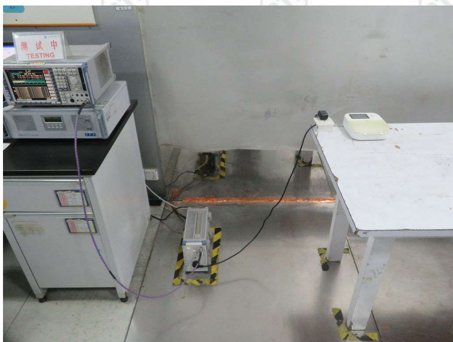
Conducted Emissions Test Setup
