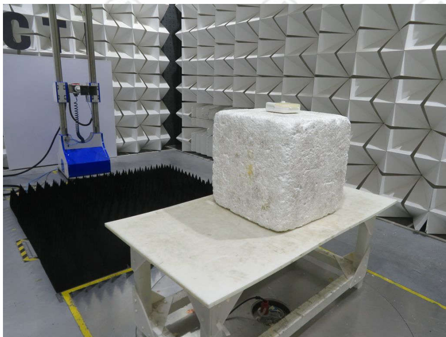
Radiated spurious emission Test Setup-3(Above 1GHz)
