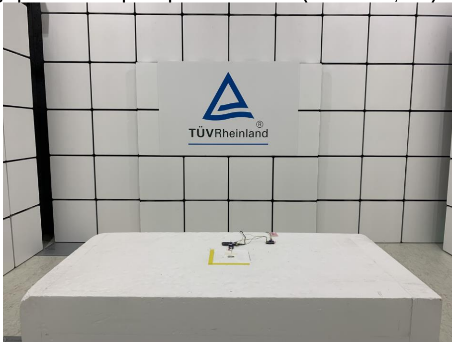
Photograph 2: Test Setup for Spurious Emissions (Front View 2, BLE)
