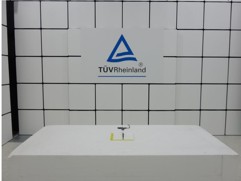
Photograph 25: Test Setup for Spurious Emissions (Front View, WiFi)
