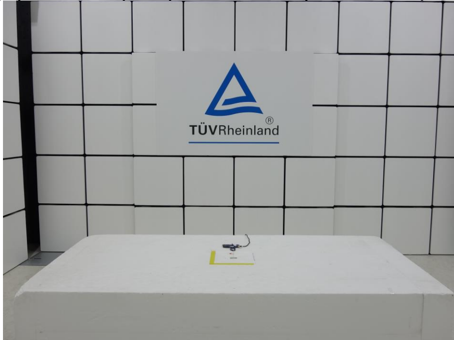
Photograph 10: Test Setup for Spurious Emissions (Front View 2, WiFi)
