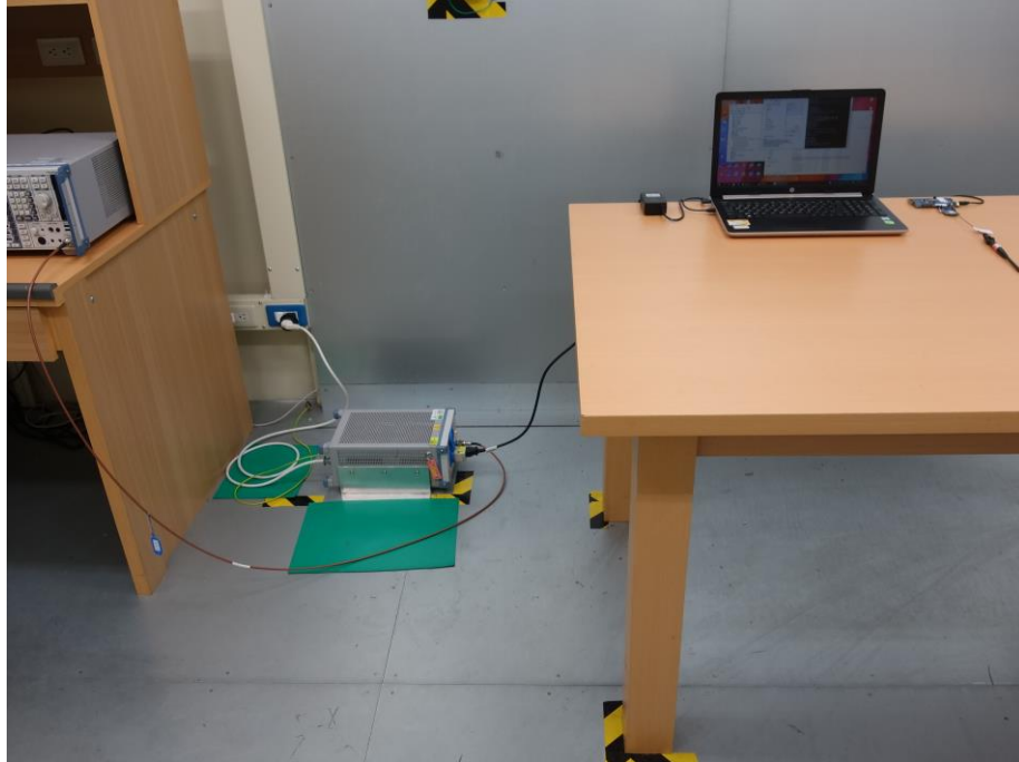
Photograph 31: Test Setup for Mains Conducted Emissions (Front View, WiFi)
