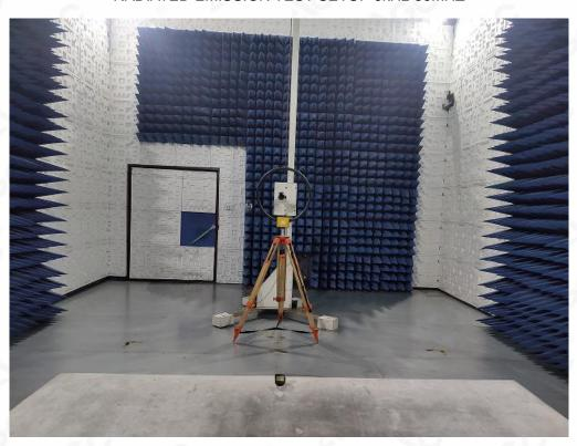
RADIATED EMISSION TEST SETUP 30MHz-1GHZ
