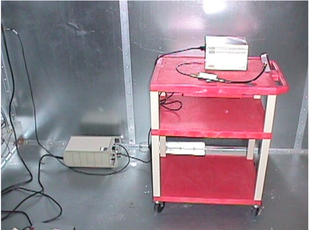
View of the Waverider NCL 1000 module during conducted emission testing.
