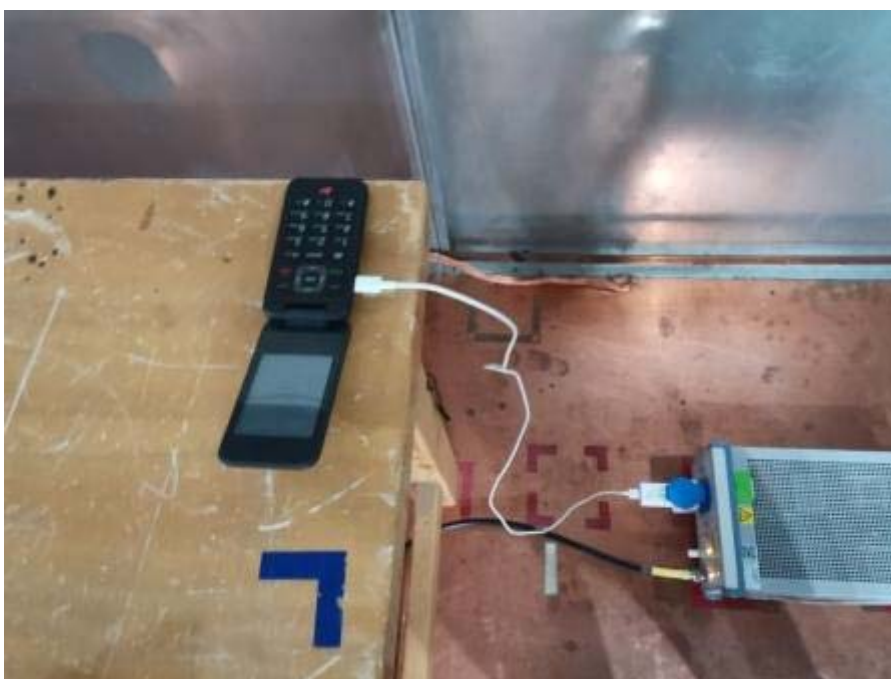
Conducted Emissions Test Setup (with charger)
