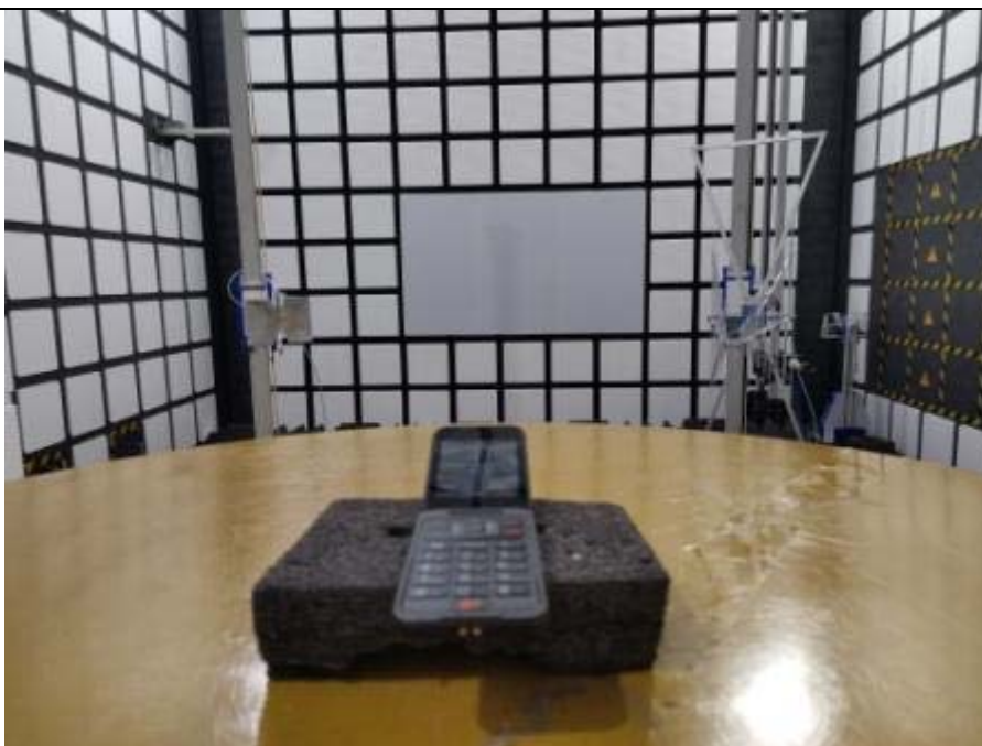
Spurious Radiated Emissions Test setup
