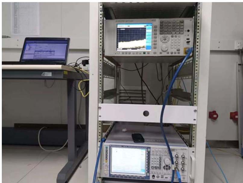
'RF Conducted Test setup (GSM/WCDMA/LTE)
