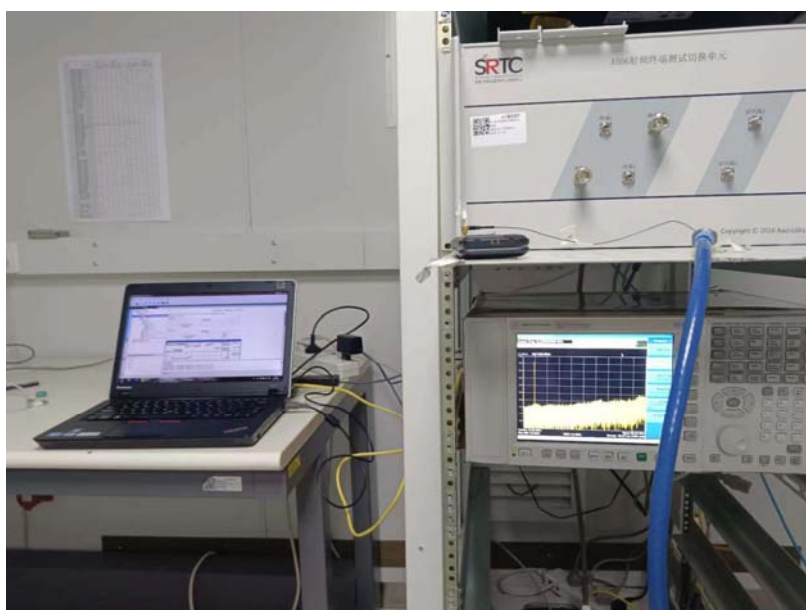
RF Conducted Test setup (BT/WIFI)
