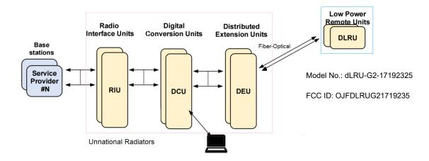
The matched units RIU/DCU/DEU are unintentional radiators, the fiber used to connect dLRU, DCU and DEU.
