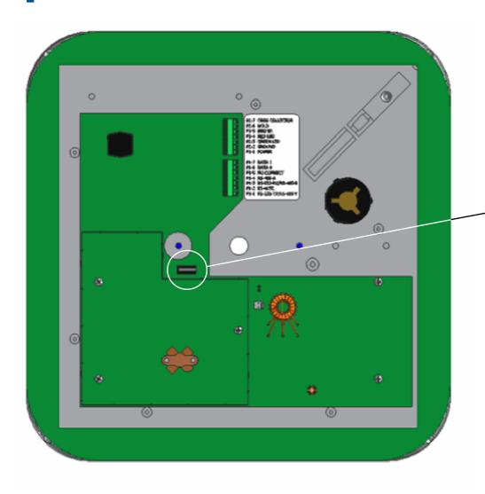
An on board tamper switch is wired through the "I'm Alive" feature and if active, the standard supervisory signal will stop if the cover is removed.
