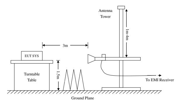
Frequency:9kHz-30MHz Frequency:30MHz-1GHz Frequency: Above 1GHz RBW=10KHz, RBW=120KHz, RBW=1MHz, VBW = 30KHzVBW=300KHz VBW=3MHz(Peak), 10Hz(AV) Sweep time= Auto Sweep time= Auto Sweep time= Auto Trace = max holdTrace = max holdTrace = max holdDetector function = peak Detector function = peak, QP Detector function = peak, AV
