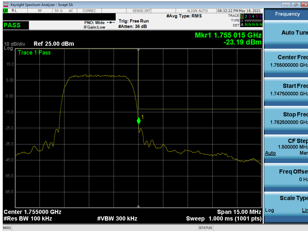
Plot 7-112. Upper Band Edge Plot (WCDMA AWS – Ch. 1513)
