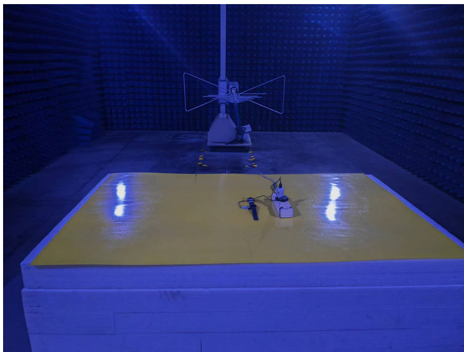
Photo of Radiated Emission Measurement (Below 1G)
