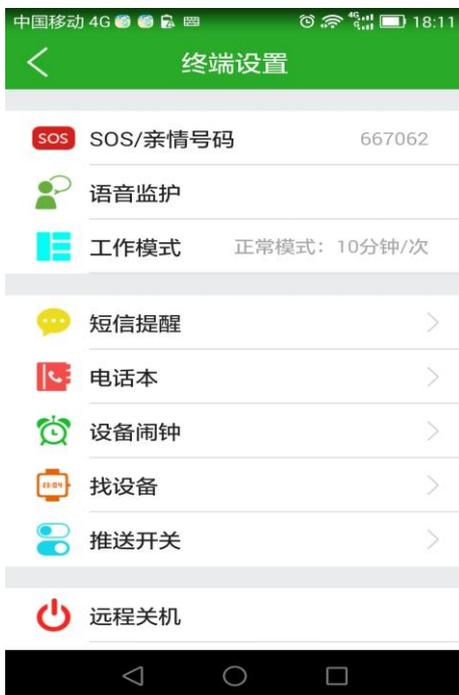
① Setting the SOS number.: You can add 3 SOS numbers on the GPS tracker. It will start to alarm and call the 3 SOS numbers in cycle after pushing the SOS button for 3seconds. If no answering, it will keep calling the 3 SOS numbers for 2 rounds.
