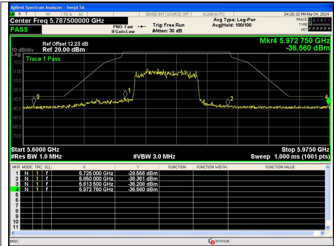
Out Of Band Emission IEEE 802.11ac_Channel 155_80MHz_Antenna 0
