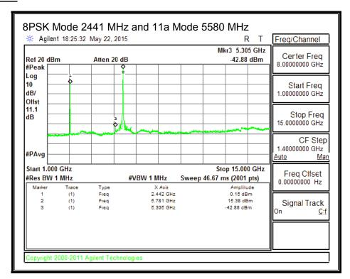
"For the co-located test, no other emissions were found after being investigated from the conducted measurement with all different combination frequencies between BT & 5GHz bands."
