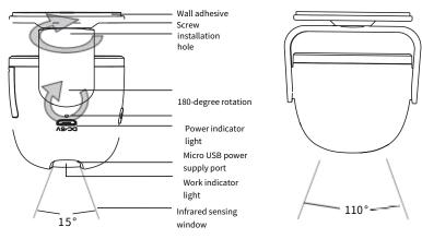
Sensing Angle: Vertical direction: 110°, horizontal direction: 15°
