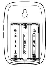
As shown in the picture, the battery cover of the receiver is pushed open from top to bottom
