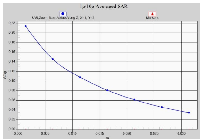
Fig. 1-3 Z-Scan at power reference point (WCDMA850)
