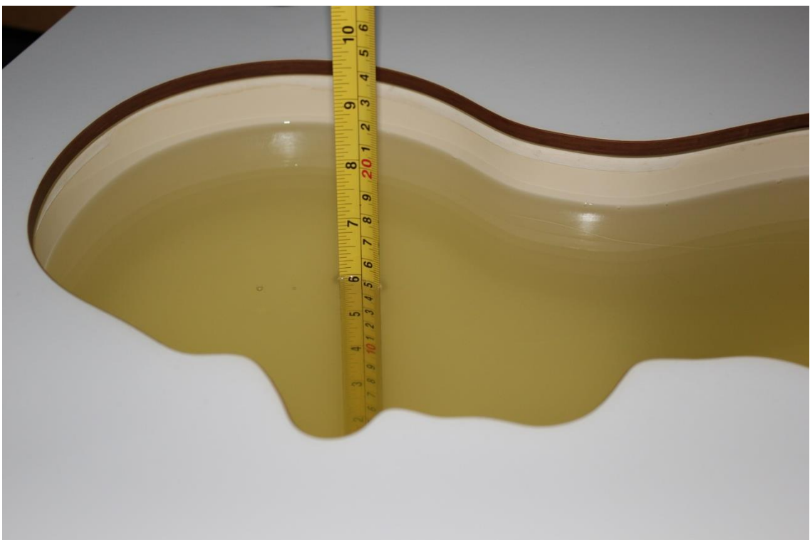
Picture 7-8 Liquid depth in the Head Phantom (2300 MHz Head)
