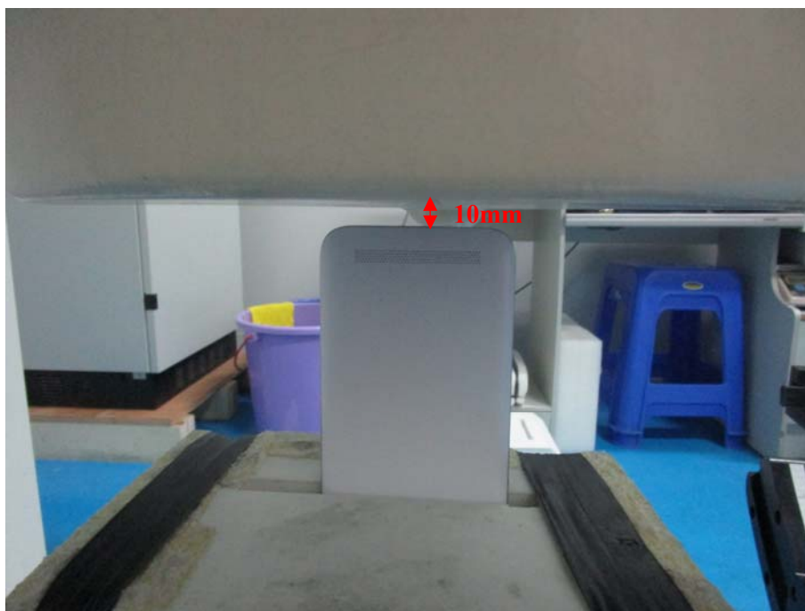
Body-worn Bottom Setup Photo
