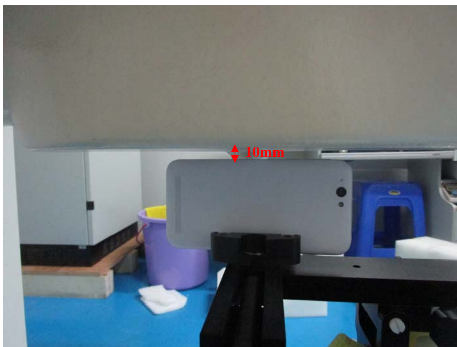
Body-worn Right Setup Photo
