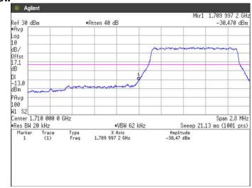
QPSK, BW 1.4MHz, RB6-0 Channel: High\_
