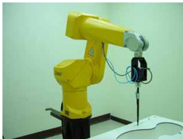
Fig. 5.2 Probe setup on robot
