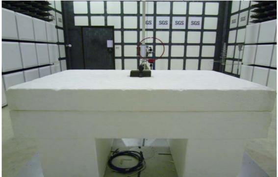
Radiated Emission Set up Photos (Below 1GHz)
