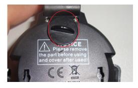
The NOTICE as shown on the above photo with white square surrounded was used to remind the user on the use of charging port cover as circled in red.
