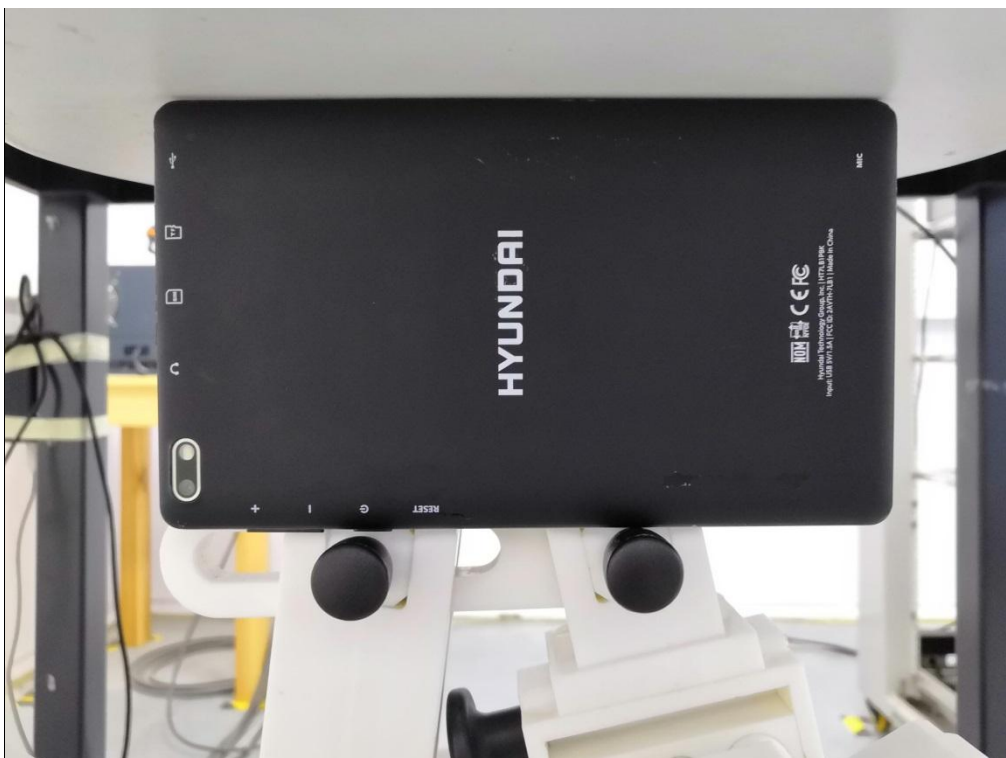
0mm body-worn Left Side Setup Photo(hotspot)
