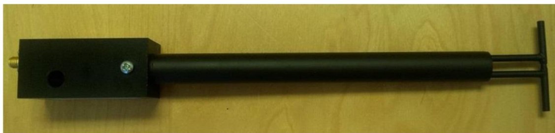
Figure 1 – MVG COMOSAR Validation Dipole
