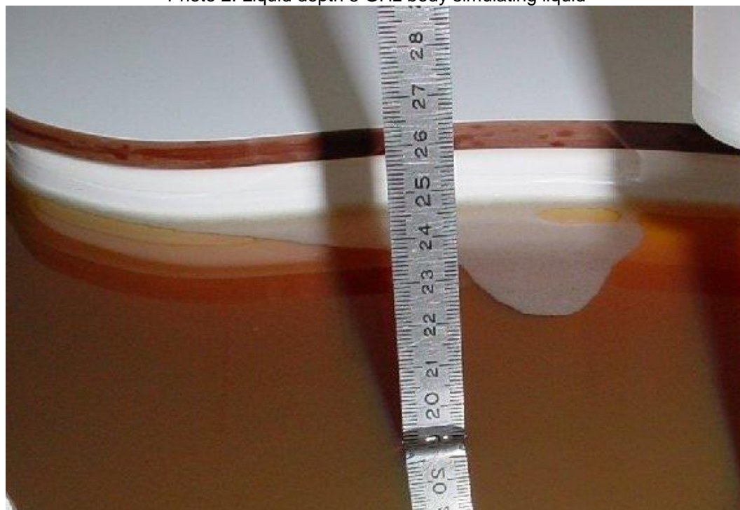
Photo 2: Liquid depth 5 GHz body simulating liquid
