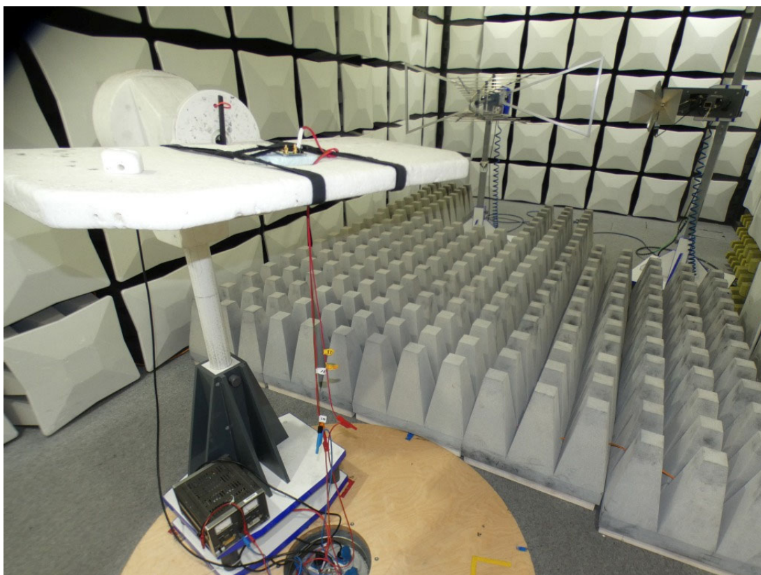
Photo 3: Test setup for radiated measurements above 1 GHz
