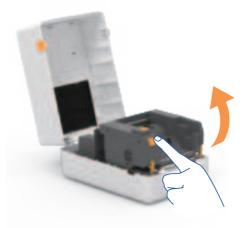
2 Remove the ribbon cassette bracket: Press the button shown to remove the bracket.
