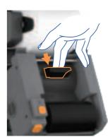
3 Remove the receiving end (A) and (B) of the ribbon cartridge from the holder.
