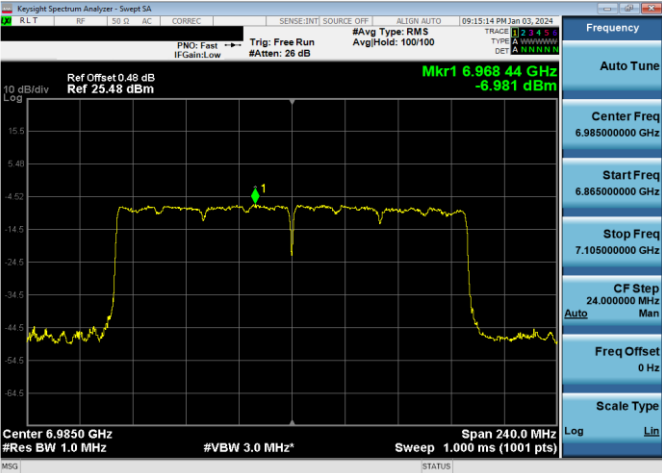
Plot 7-863. LPI Power Spectral Density Plot SDM Antenna WF2a (160MHz 802.11ax RU996x2 (UNII Band 8) – Ch. 207)
