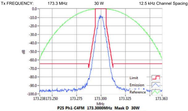
P25 Ph1-C4FM 173.3000MHz Mask D 30W RBW=100Hz, VBW=1000Hz, Detector Mode=Peak Result=Pass
