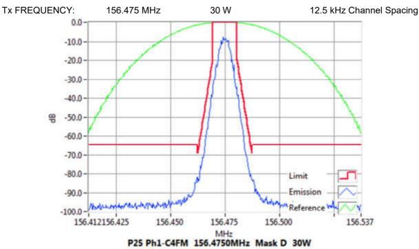
P25 Ph1-C4FM 156.4750MHz Mask D 30W RBW=100Hz, VBW=1000Hz, Detector Mode=Peak Result=Pass
