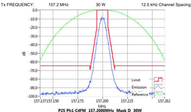
P25 Ph1-C4FM 157.2000MHz Mask D 30W RBW=100Hz, VBW=1000Hz, Detector Mode=Peak Result=Pass
