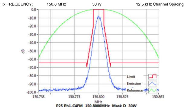
P25 Ph1-C4FM 150.8000MHz Mask D 30W RBW=100Hz, VBW=1000Hz, Detector Mode=Peak Result=Pass
