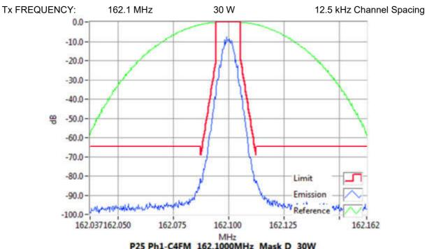
P25 Ph1-C4FM 162.1000MHz Mask D 30W RBW=100Hz, VBW=1000Hz, Detector Mode=Peak Result=Pass
