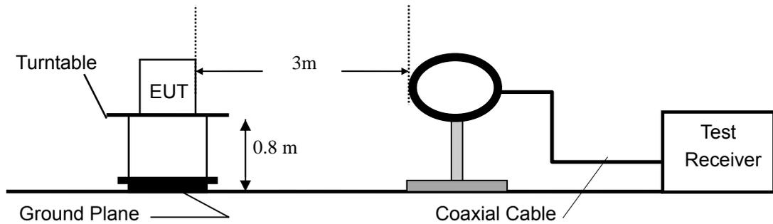
Radiated Emission Test Set-Up, Frequency Below 1GHz
