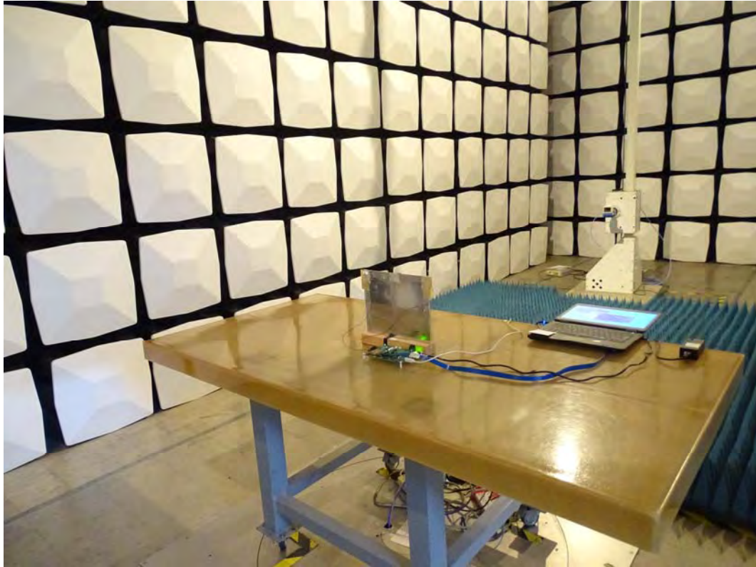
Back View of Radiated Test (Horn)
